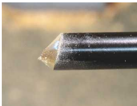
▲ Pic.1 The 6mm bowl gouge is made from 10mm steel. I prefer this tool for all my finishing cuts. I grind it at about 45° and never put a long grind on it as the flute will clog up quickly if it is used for pull cuts
